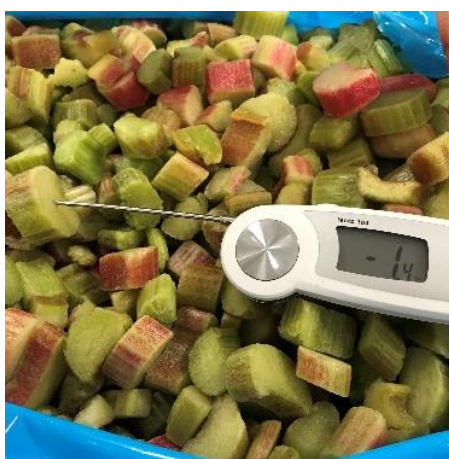
Rhubarb 10 kg blocks (3 x 10 kg) 300 kg/h from -18 °C to -3 °C/-1 °C
