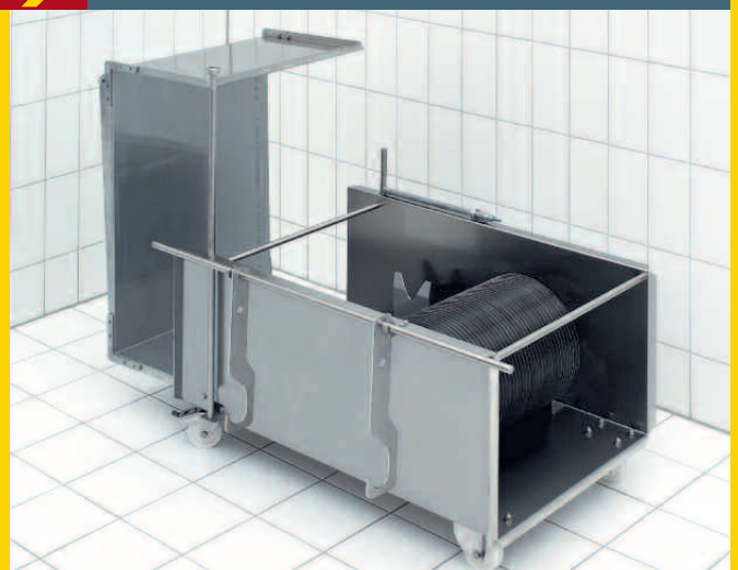
Cleaning wagon for 2 blade shafts (cover open, lift-out-device hung in)
