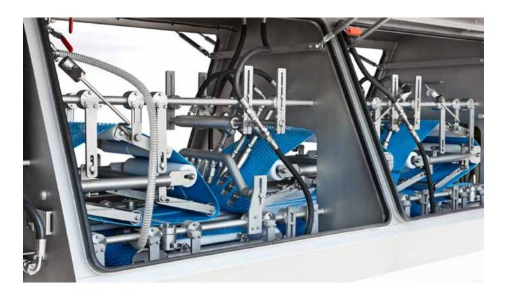
Water is an efficient and gentle way to de-scale a fish. The De-scaler 800 uses water pressure to gently de-scale the fish without damaging meat, eyes, or gills. At the same time, the use of water is an efficient bacteria remover, reducing listeria greatly on the surface of the fish and ensuring a clean fish and a clean processing line without compromising the average through-put time.
